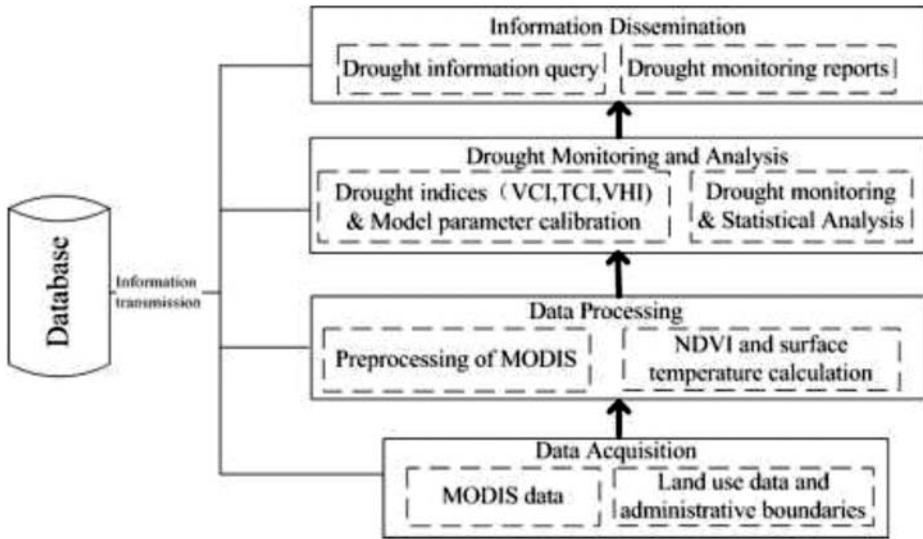
Figure 1. A configuration of the DroughtWatch system.
